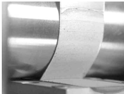
FIGURE 13 Aluminium peel arm 152 \mu\text{m} thickness not conforming to the mandrel of radius 15 mm.
